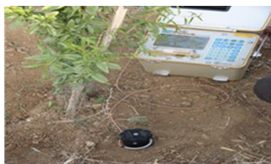
Fig. 3- Measurement of volumetric moisture of treatments by TDR device
