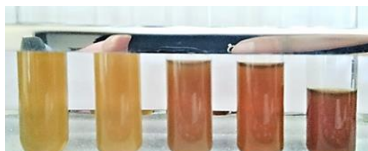
Fig. 4. Color change by reducing the amount of extract from 5 to 1 ml (left to right).
