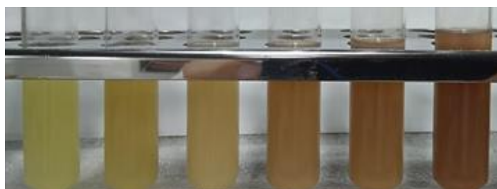
Fig. 3. Color change due to increased pH (left to right) in the extract solution and silver nitrate.
