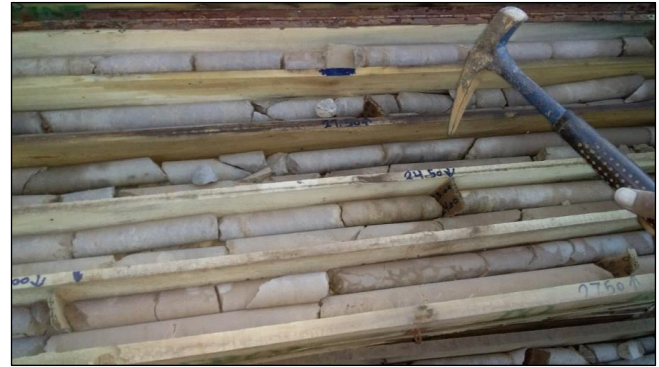
Fig. 7. Intact cylindrical core samples collected from the Tajkuh lead–zinc mine
