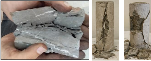
Fig. 9. Representative failure patterns of intact rock specimens after laboratory compression testing
