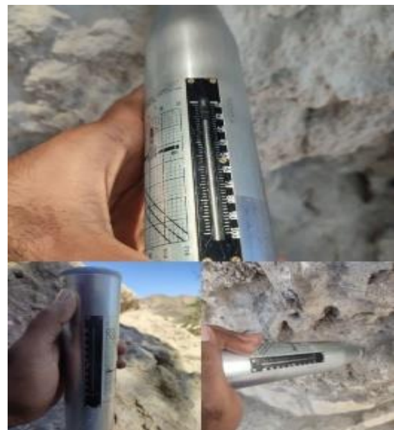
Fig. 5. Schmidt Hammer test
