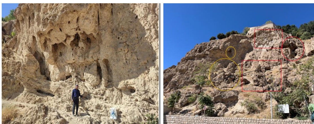
Fig. 2. The figure displays caves formed by the weathering and erosion of impurities and soft materials, with evidence of clay and sand presence observed.
