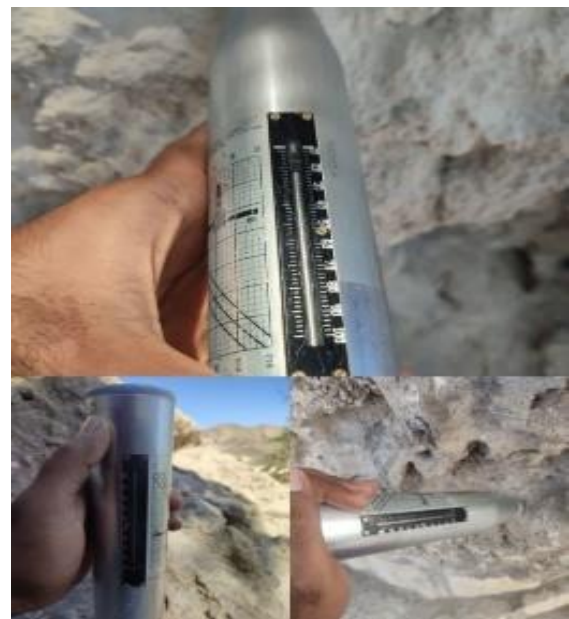
Fig. 5. Schmidt Hammer test
