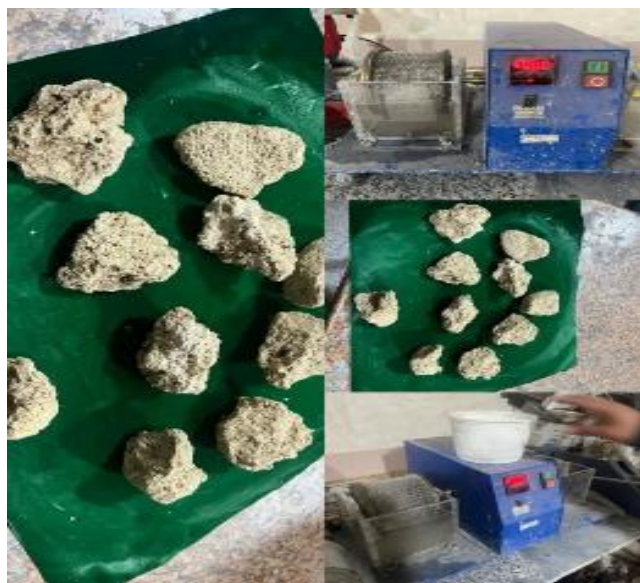
Fig. 6. Slake Durability test for rock
