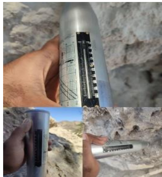
Fig. 5. Schmidt Hammer test
