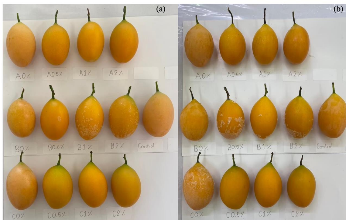
Fig. 4. Appearance of marian plums alone (control) or treated with edible coatings at varying beeswax concentrations (0%, 0.5%, 1%, 2%); A: carboxymethyl cellulose-beeswax coatings, B: starch-beeswax coatings, and C: chitosan-beeswax coatings. The fruit were stored at 10^\circ\text{C} at day 0 (a) and after 16 days of storage (b).
