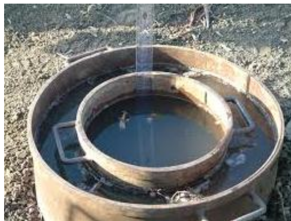
Fig. 3. Measuring the infiltration by double-ring method
