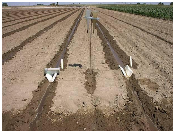
Fig. 4. Measuring the infiltration by the Input-output furrow method
