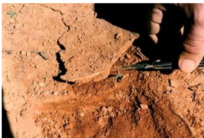
Fig. 1. A thin surface crust caused by raindrop impact on a bare soil with poor structure.
