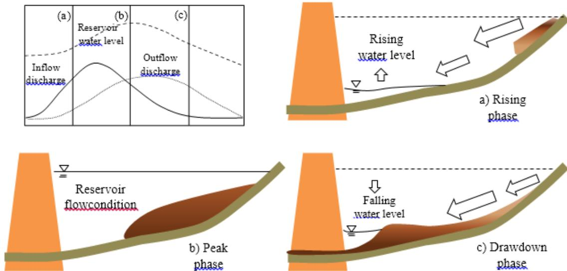
Fig. 1. Conceptual schematic view of the sediment transport process within the FMD.
