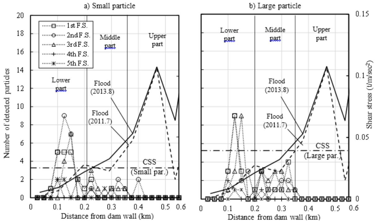
**Fig. 5.** Variation of the maximum shear stress in respect to both the distance from the FMD and the critical shear stress (CSS) for a) small particles; b) large particles.
