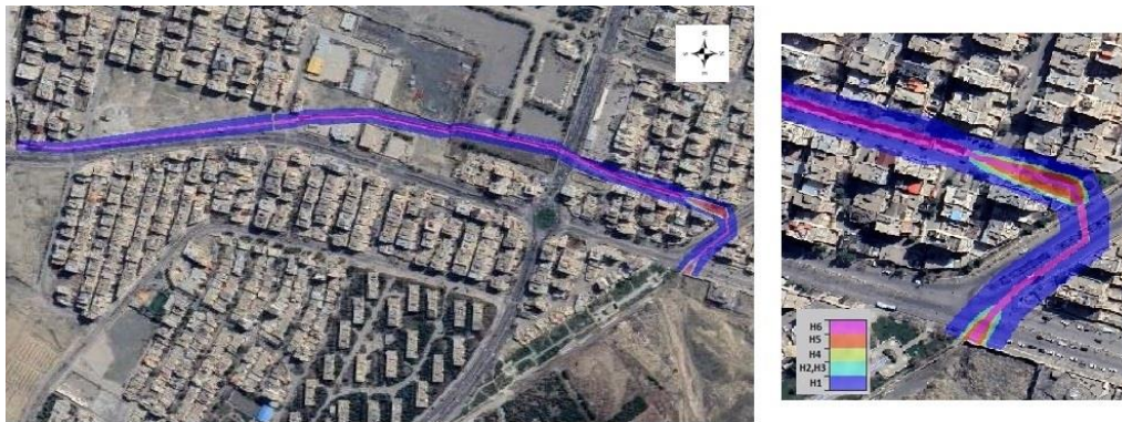
Fig 10. Flood hazard zoning map of Ladan watercourse based on Code 821 for a 100-year return period flood.
