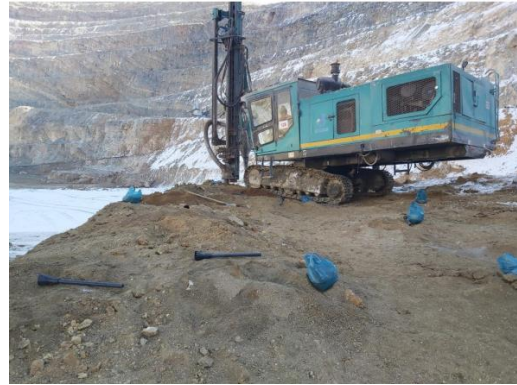
Fig. 11. The drilling rig and Power Dock spacers in the explosive block 2760-32
