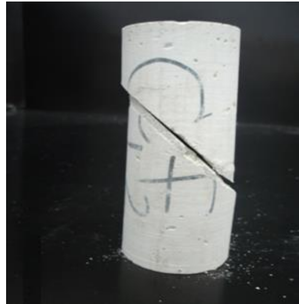
Fig. 6. Failure along the discontinuity-infill material interface for stronger infill materials. The discontinuity is oriented at 45°.
