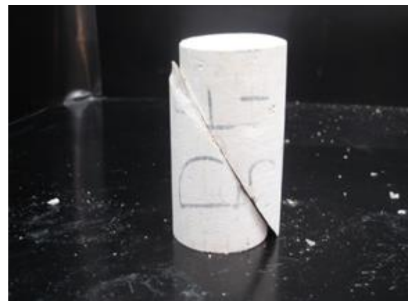
Fig. 7. Failure along the discontinuity-infill material interface for stronger infill materials. The discontinuity is oriented at 60°.
