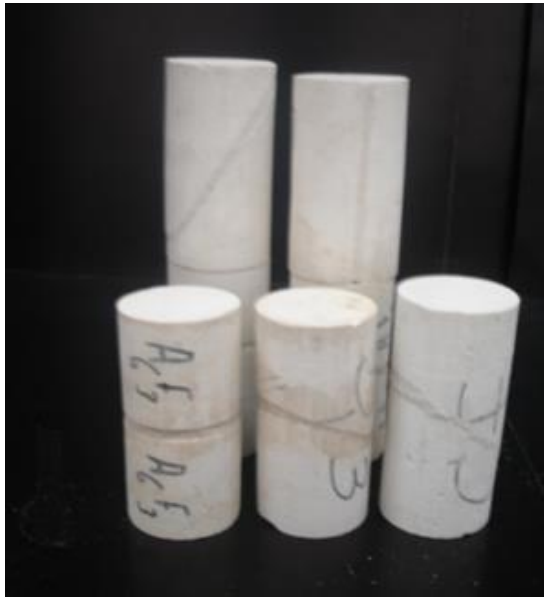
Fig. 3. Specimens with discontinuities at different orientations upon filling with the model infill materials.
