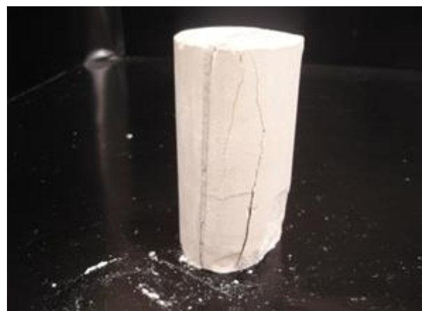
Fig. 8. Failure in the intact body of the specimen with an infilled discontinuity oriented at 90°.
