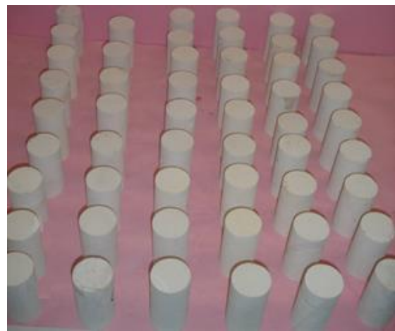
Fig. 1. A group of specimens prepared based on the standard defined by the International Society of Rock Mechanics (ISRM) (1979)
