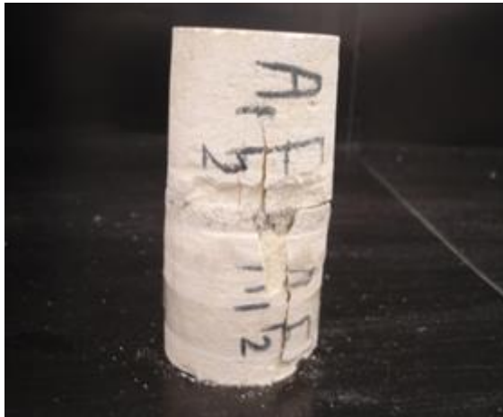
Fig. 4. Failure in the intact body of the specimen with a discontinuity oriented at 0°.
