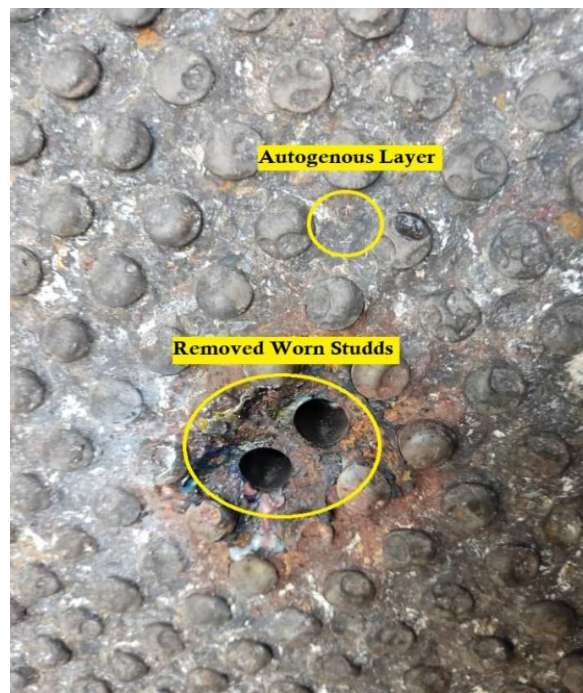
Fig. 5. An image of the removed worn studs and the autogenous wear protection layer
