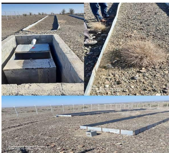
Fig. 2. Erosion plots of Dehgin watershed; Pay attention to the two cubic meter tank and the surface covered by the armor of these plots
