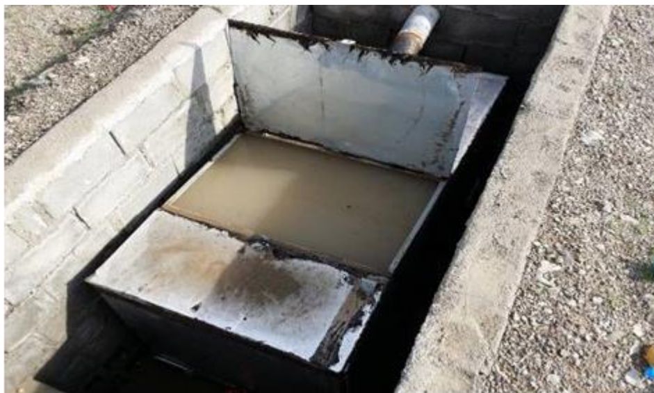
Fig. 6. The filling of one of the 2000-liter tanks of the erosion and sedimentation plots in the Dehgin Basin after rain
